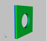
Using the Difference operator on multiple objects is handy in this case—otherwise you would need to insert and the cutter multiple times.
