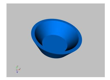
Creating an extruded object is nearly the same. Select Object→Insert Object→Extrusion. A dialog similar to the Create Revolved Surface dialog will be shown (omitted here to save space). The main difference is that you must input the extrusion *length* rather than an angle.
