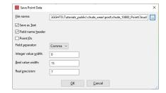
You may save the data as a CSV (default), DAT, OBJ, PLY, STL, VTK, or VTP file. By default, the output is written as ASCII text. You can also save PLY, STL, VTK, and VTP files in binary format by unchecking the Save as Text option.
