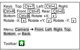
The ("Home") button on the Toolbar can also be used to undo all edits, reset the zoom level, and reset the camera to the front view.
